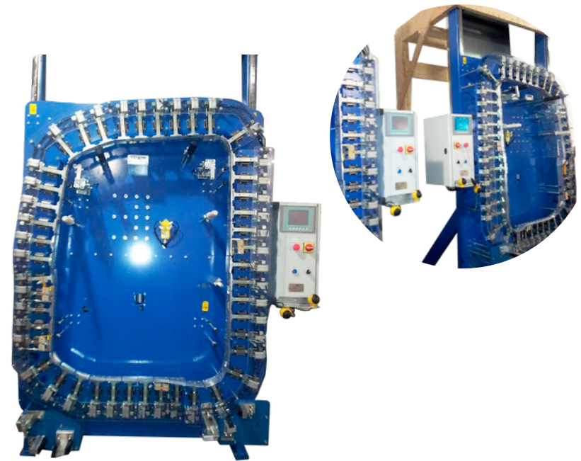
MOUNTING THE RUBBER ON THE DOOR
